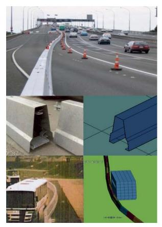
The simulation model is based on LS-DYNA Finite Element software. A design-of-simulations was developed and carried out to determine the optimum design parameters. On basis of the analysis, a new design shape was proposed that has a performance comparable with the one of competition. The developed design tool can be used to simulate future designs of safety barriers, or predict outcome of actual crash tests.
