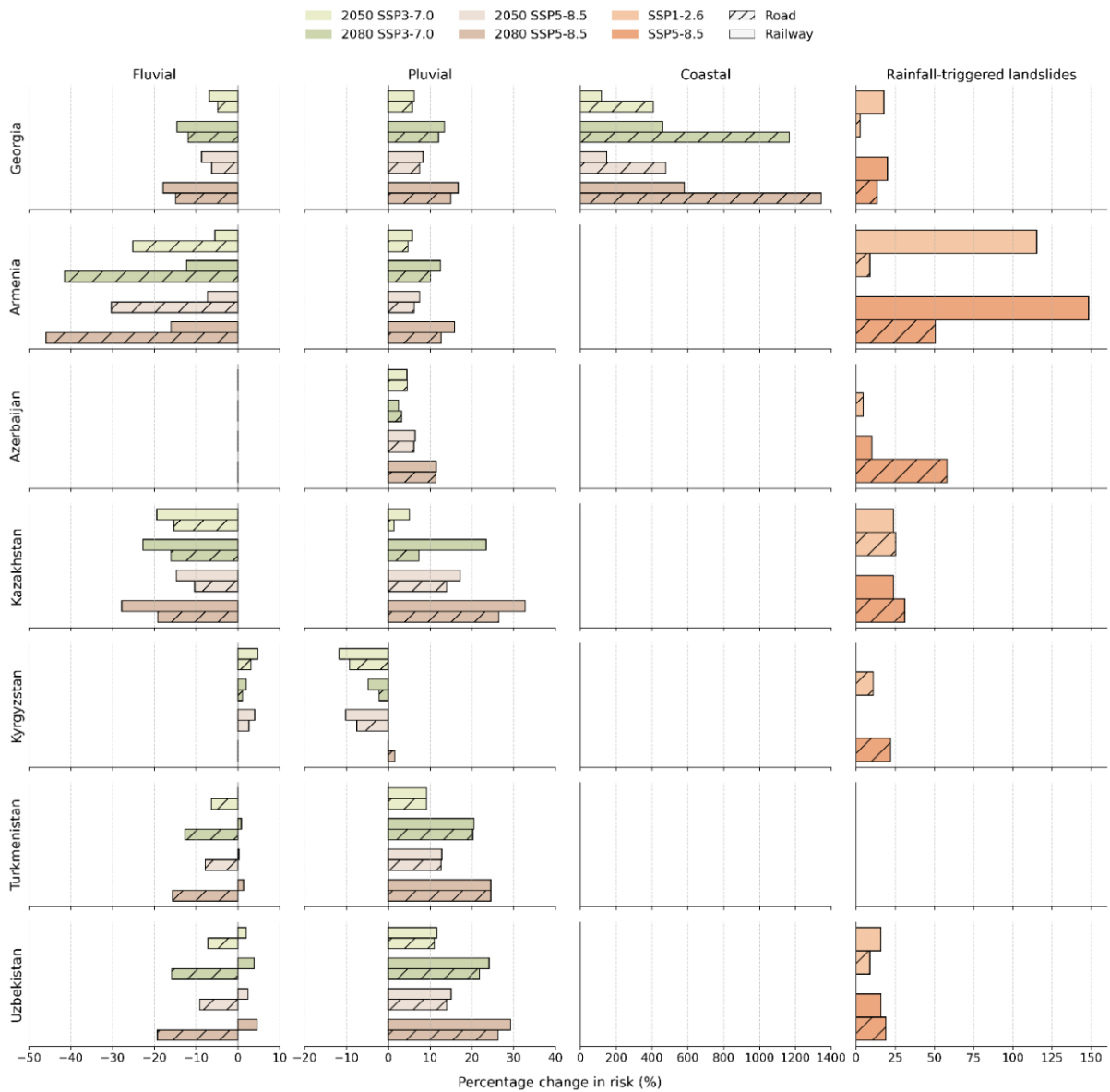
Figure 2. The relative change (%) in road and rail risk for the MC due to fluvial, pluvial, and coastal flooding, as well as rainfall-triggered landslides, across Middle Corridor countries under various future climate scenarios.
