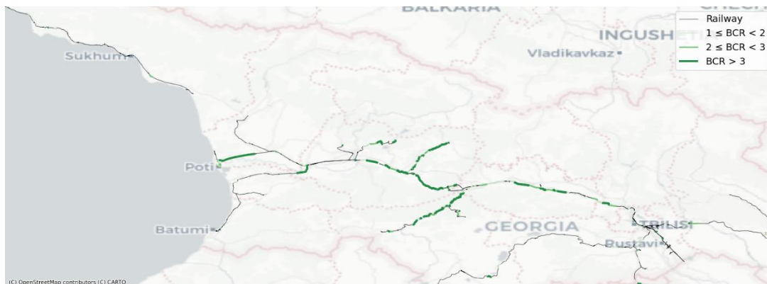
Figure 3. Spatial distribution of railways in Georgia prioritized for improvement based on economic viability, assuming an investment of 3% of the construction costs, 6% discount rate and a lifetime of 15 years.
