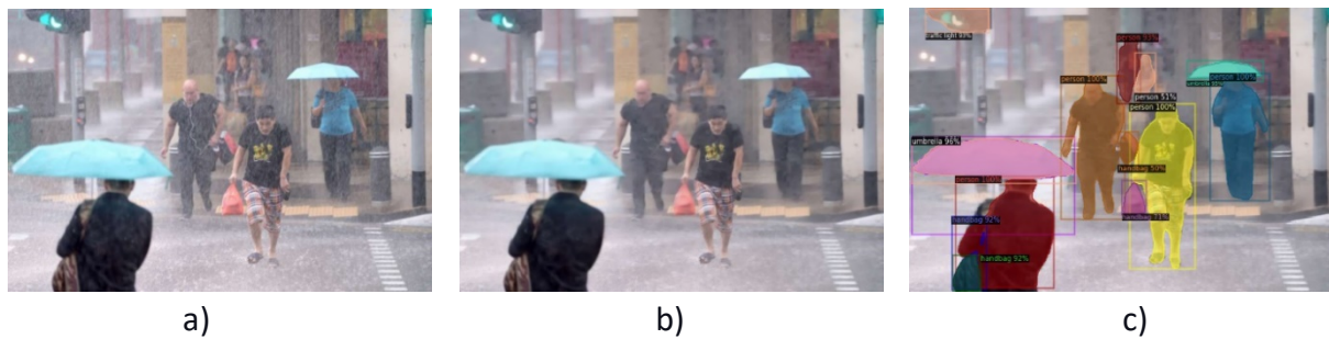
Fig. 4. Project 4: vision enhancement system. a). The original captured image; b) The enhanced image via AR; c) Object detection and classification.
