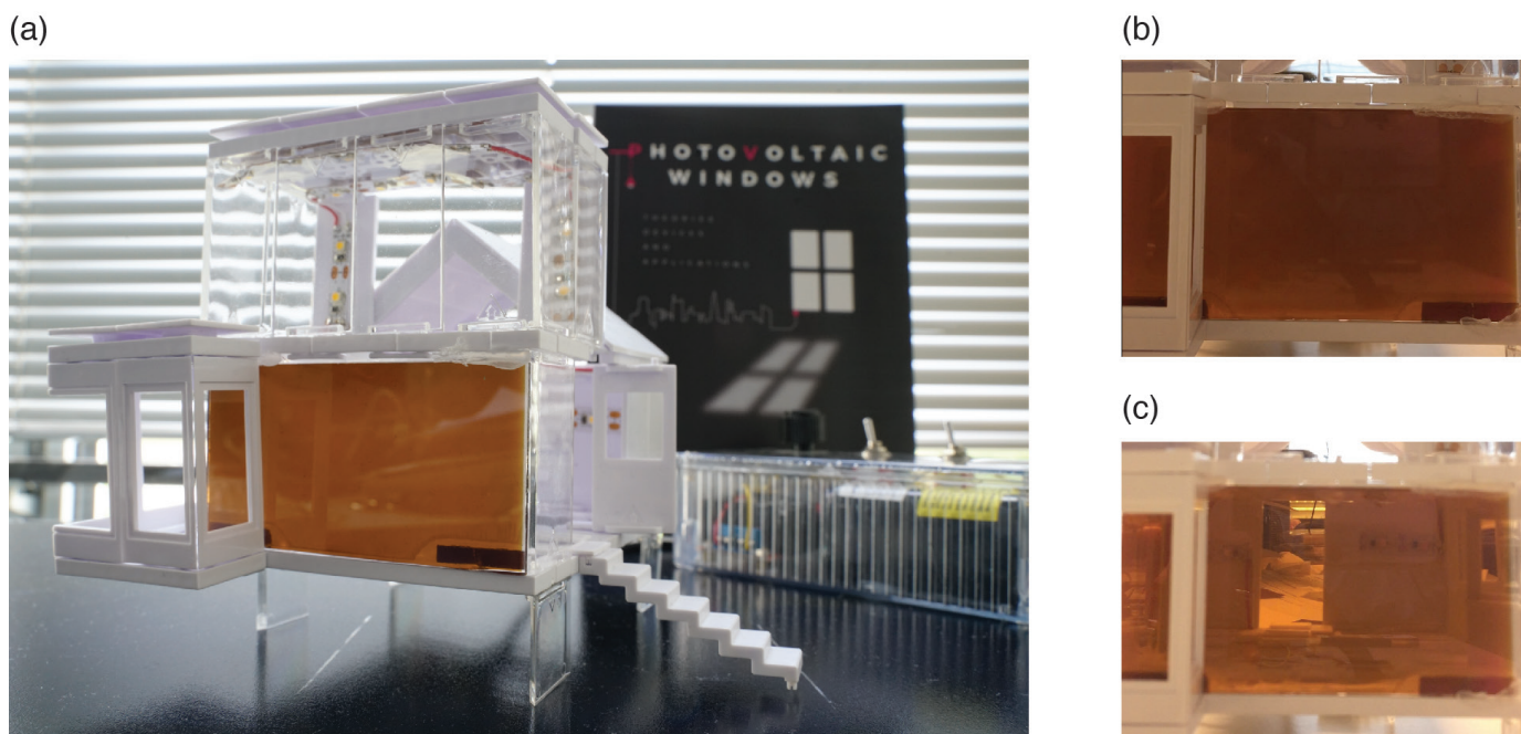
(a) A demonstration house model of STPV-PDLC system. The window dimensions are around 10 * 5 cm. (b) The STPV-PDLC window reveals opaque in the 'off' state when no voltage is applied to the PDLC film. (c) The STPV-PDLC window turns semi-transparent when an AC voltage is applied to the PDLC film
