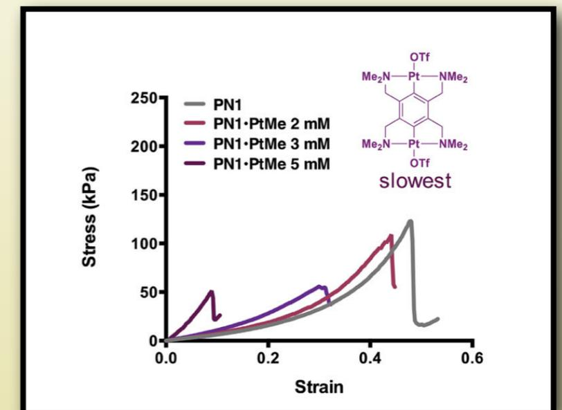
The “slow” (intermediate) linkers increase the strain-at-break and the toughness
