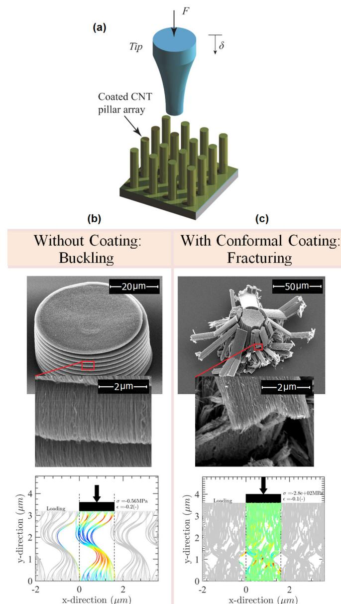
**Figure 2.** Mechanical compression of CNT's (a) Flat-punch nano-indentation on a vertically aligned a CNT pillar, (b) Smooth localized micro buckling on CNT pillar, (c) Fracturing deformation on a CNT pillar with 10.5 nm a-SiC coating; Image adapted from [3]
