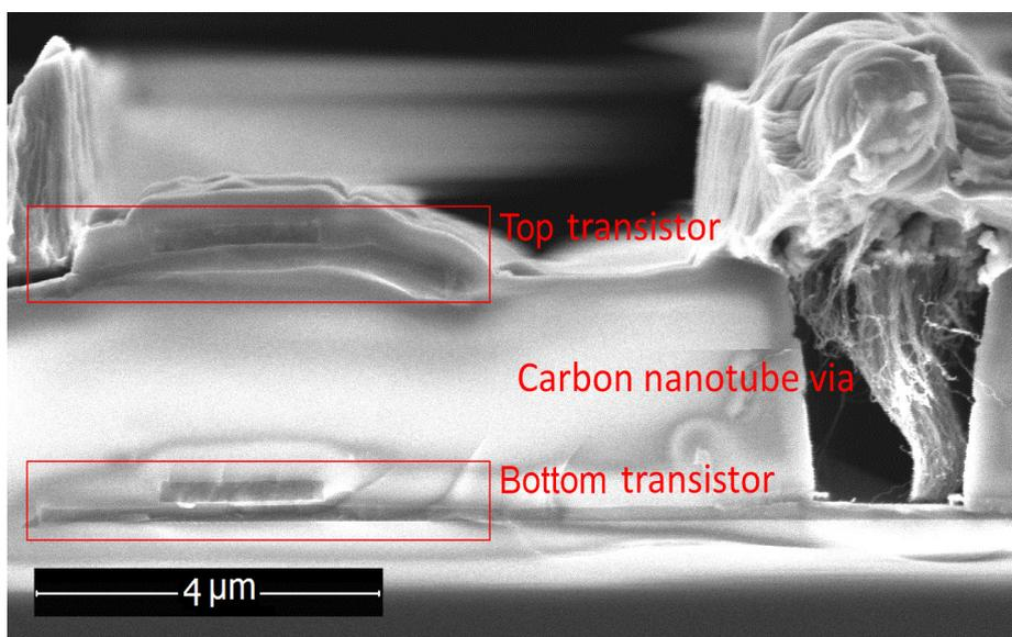
Figure 5. Wafer containing the 3D devices: cross-section of two-layer showing the active areas and CNT via; Image adapted from [7]
