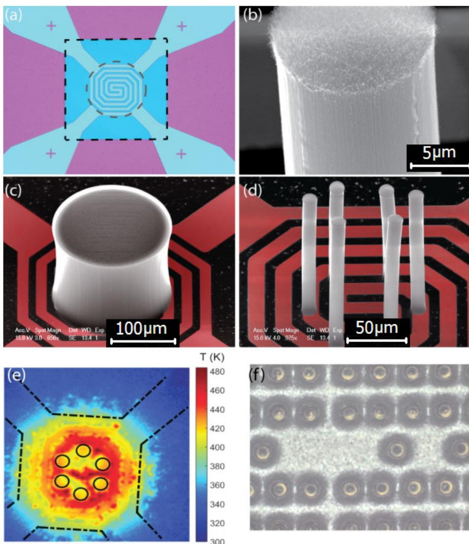
Figure 3. CNT array synthesized on top of the suspended MEMS structure. (a) MEMS structure that can be heated up by Joule heating. (b) Tip of a high aspect ratio CNTs; (c) CNTs structure called single micropin; (d) Multi-pin configuration. (e) Infrared thermal maps of the micropin configuration. (f) Thermal interposer made of coated high aspect ratio CNTs integrated in epoxy molding compound; Image adapted from [4] and [5]
