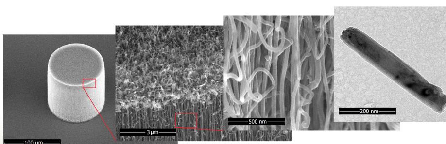
Figure 6. Coated CNT pillar as a superconductor interconnect
