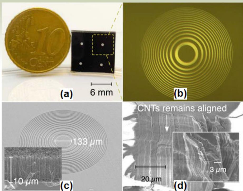
Figure 4. (a) Fabricated stretchable Fresnel lens containing  $2 \times 2$  lens units, (b) Optical microscope image of one lens, (c) Tilted SEM image of the diffractive CNT pattern, the inset shows a close up view of the vertically aligned CNT, (d) SEM image of the CNT with the PDMS percolated thoroughly into the CNT bundles; Image adapted from [6]
