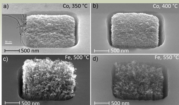
**Figure 1.** Holes filled with CNTs grown at different catalysts and temperatures: (a) Co, 350 °C; (b) Co, 400 °C; (c) Fe, 500 °C; and (d) Fe, 550 °C; Image adapted from [1].
