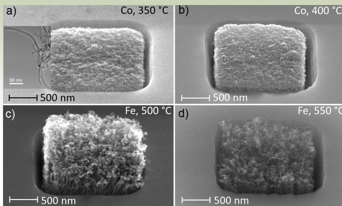
**Figure 1.** Holes filled with CNTs grown at different catalysts and temperatures: (a) Co, 350 °C; (b) Co, 400 °C; (c) Fe, 500 °C; and (d) Fe, 550 °C; Image adapted from [1].
