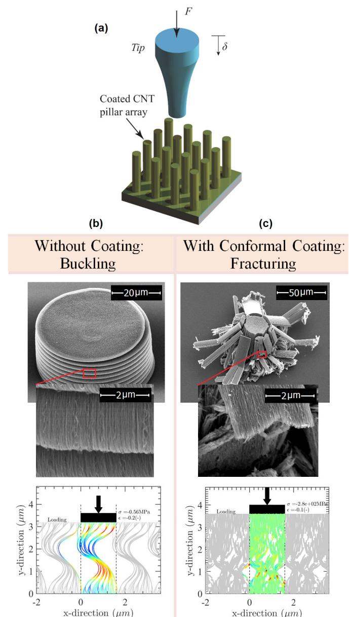
**Figure 2.** Mechanical compression of CNT's (a) Flat-punch nano-indentation on a vertically aligned CNT pillar, (b) Smooth localized micro buckling on CNT pillar, (c) Fracturing deformation on a CNT pillar with 10.5 nm a-SiC coating; Image adapted from [3]
