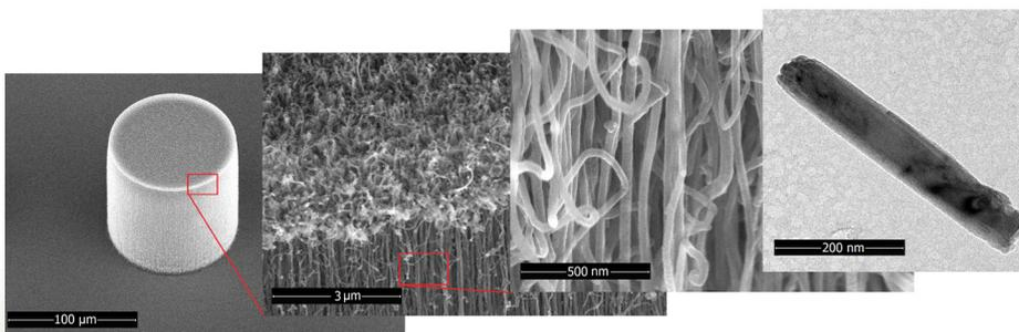
Figure 6. Coated CNT pillar as a superconductor interconnect
