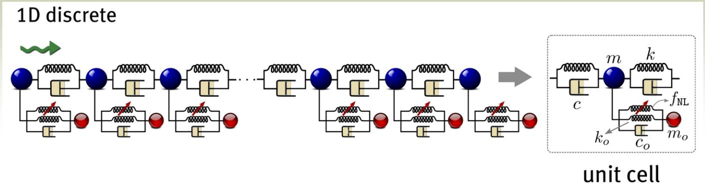
Figure 3: One-dimensional model of metamaterial with nonlinear local resonators
