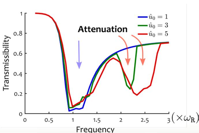
Figure 5: Transmission analysis of a nonlinear locally resonance metamaterial depicting a second attenuation zone
