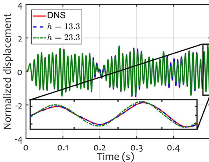
Figure 9: 1D nonlinear metamaterial transient problem analyzed via computational homogenization and direct numerical simulations. Full problem, macro and micro scales are shown. A typical solution is depicted for two levels of the amount of homogenization parameter  $h$  in comparison with solution via the conventional direct numerical simulation (DNS), with good agreement observed (8)
