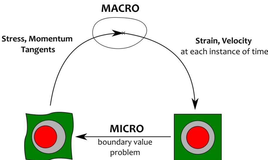
Figure 8: Scheme of dynamic computational homogenization implemented to perform transient analysis of nonlinear metamaterial
