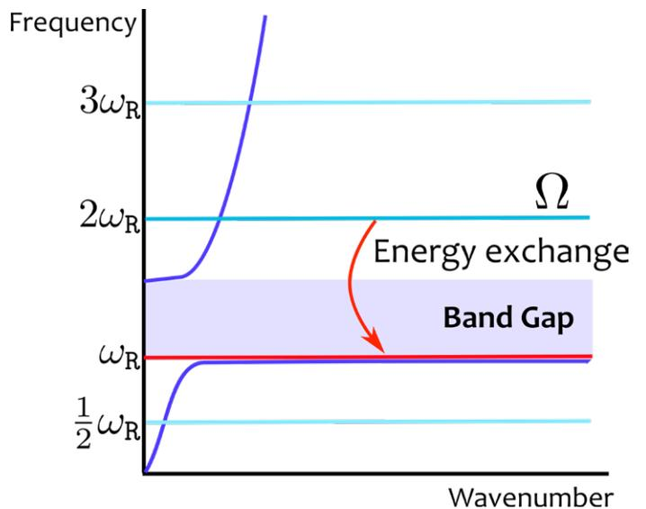
Figure 6: Scheme of the mechanism responsible for the second attenuation zone depicting energy exchange due to autoparametric resonance
