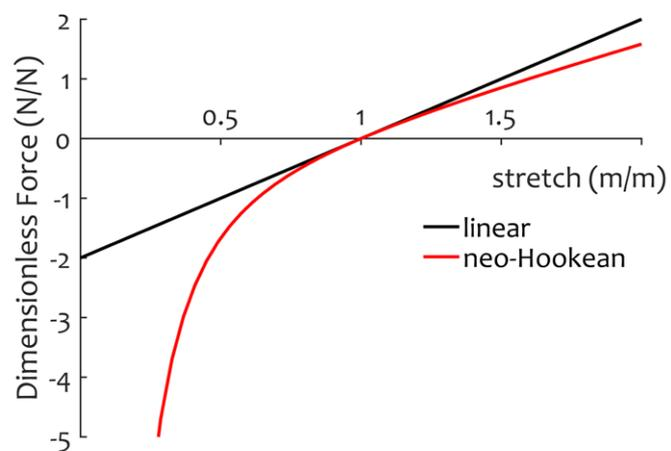
**Figure 2: Linear and nonlinear (neo-Hookean) local interaction forces versus stretch in locally resonant metamaterials**
