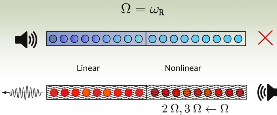
Figure 7: Nonreciprocal behavior of a structural system composed of linear and nonlinear locally resonant metamaterials connected in series and excited with frequency  $\Omega = \omega_R$
