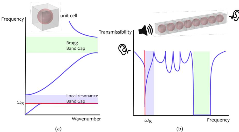
**Figure 1: Basic features of metamaterials (1D periodicity and longitudinal wave propagation): (a) dispersion diagram based on the unit cell analysis, (b) corresponding transmissibility plot ( $\omega_R$  is the local resonance frequency)**
