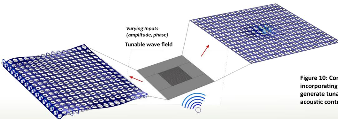
Figure 10: Conceptual scheme of a device incorporating nonlinear metamaterial able to generate tunable wave field for vibration and acoustic control
