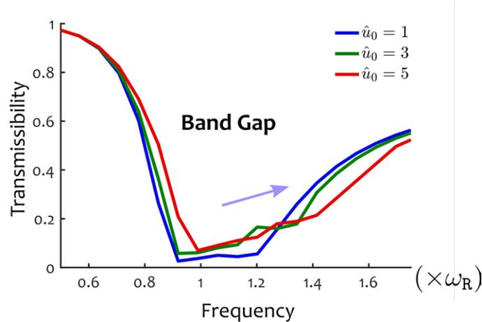
Figure 4: Amplitude-dependent transmission of a nonlinear locally resonant metamaterial: onset of tunability
