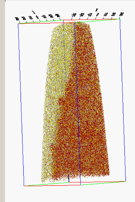
Martensite and austenite in steel (scale in nm)
