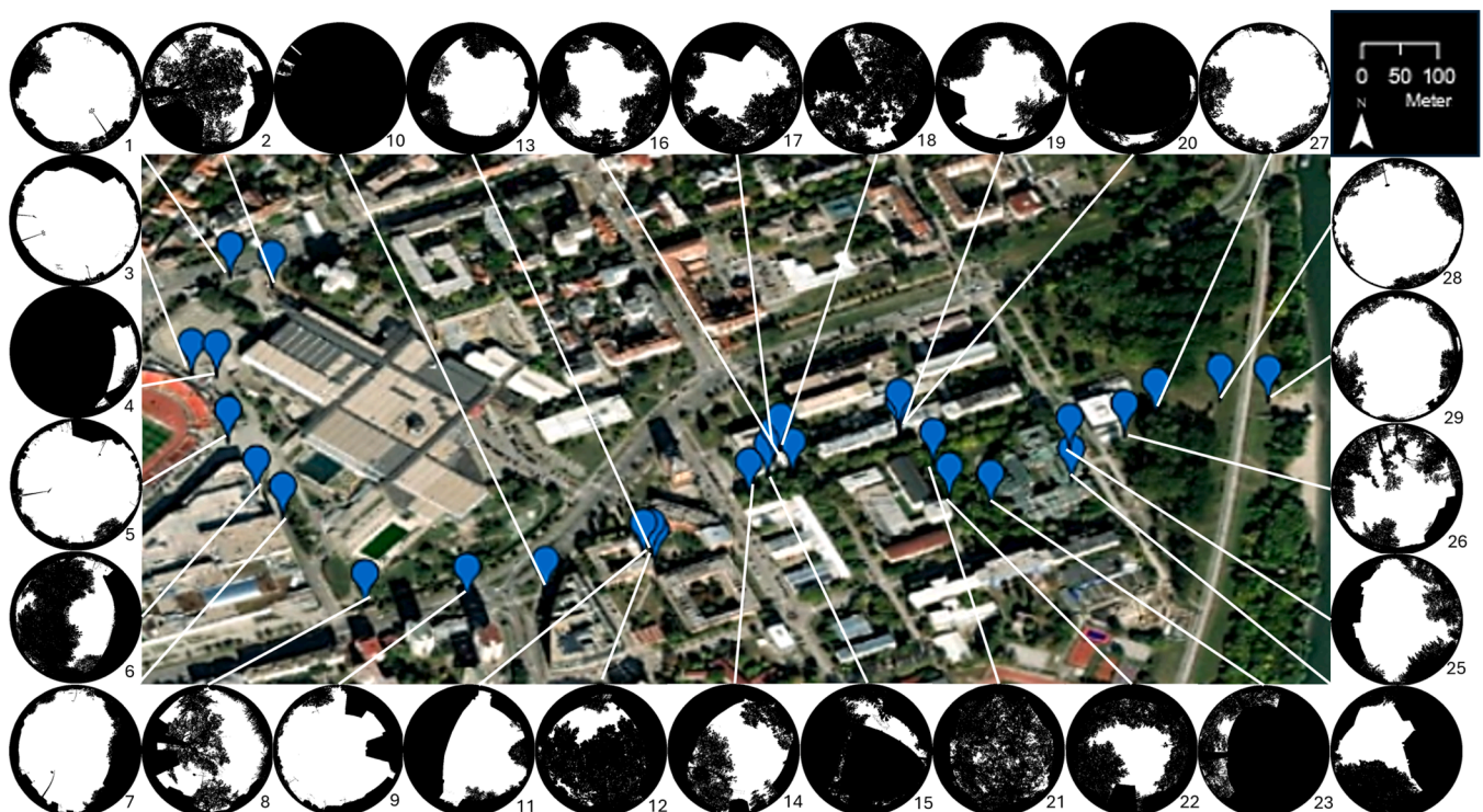
Fig. 2. Micrometeorological measurement locations and their classified fisheye lens images of the sky at each location in Novi Sad, Serbia.
