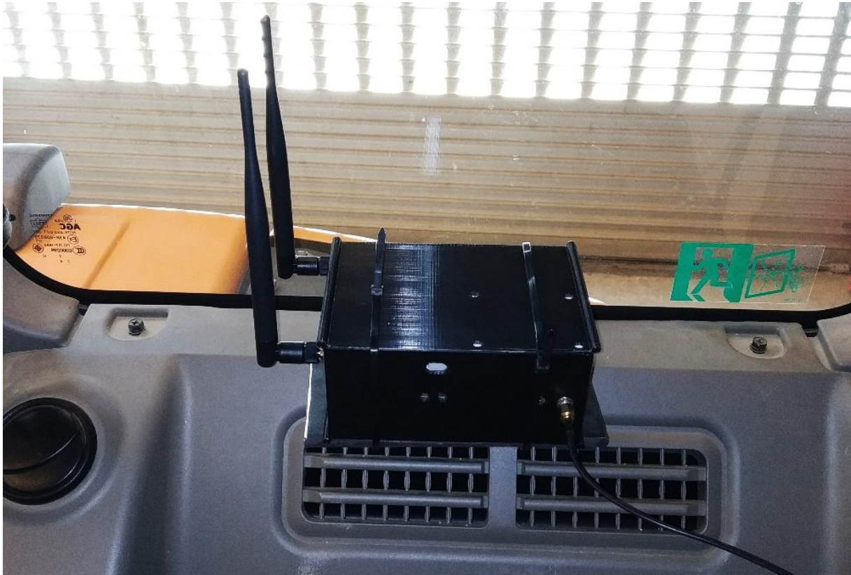
Figure 37. Central station mounted in the excavator cabin
