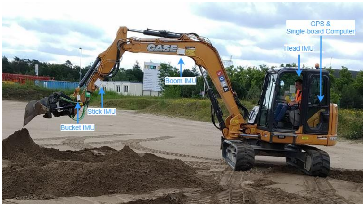
Figure 20. The configuration of the system's hardware on an excavator
