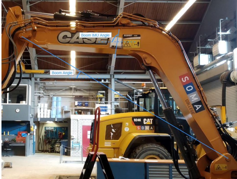
Figure 34. Inclinations of the excavator boom and the boom IMU
