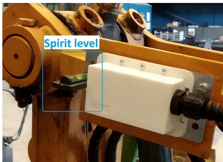
Figure 39. Bucket sensor equipped with a spirit level on its casing
