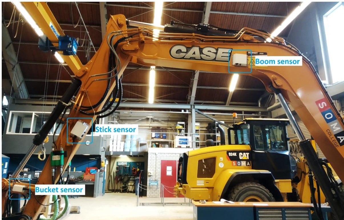
Figure 38. Sensor arrangement on an excavator
