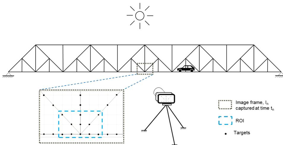
Figure 2: Schematic of a vision-based monitoring system
