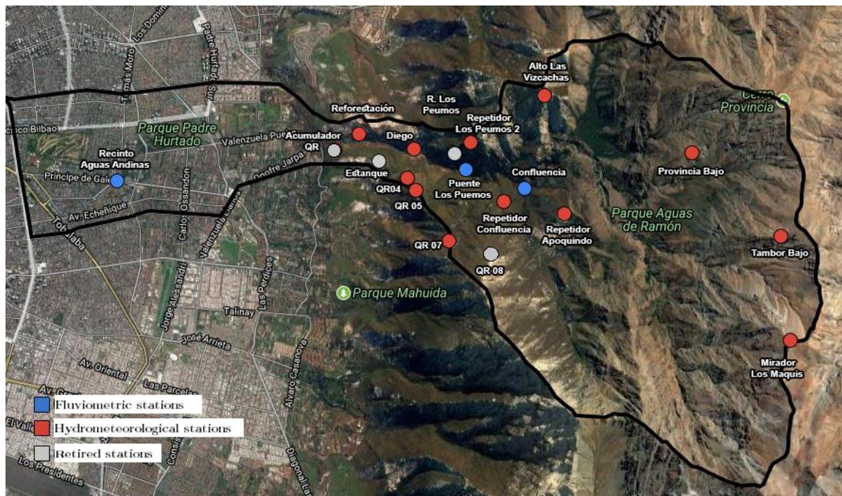
Fig. 1. Map of the Quebrada de Ramón wireless sensor network for early warning of flash floods.
