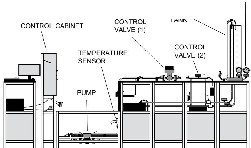
Figure 1: Test rig for resilient system design evaluation
