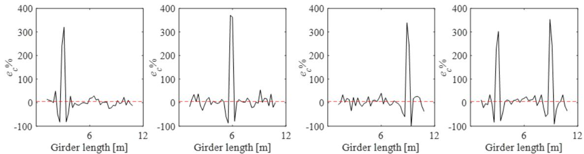
Figure 2: Damage located at several locations in the girder of 12m. the noise in this scenario is aggregated from the maximum noise level ( $N_1$ ) with the scaling effects from  $F_1$ . The red dashed lines indicate a 5% damage threshold above which damage is said to be present.
