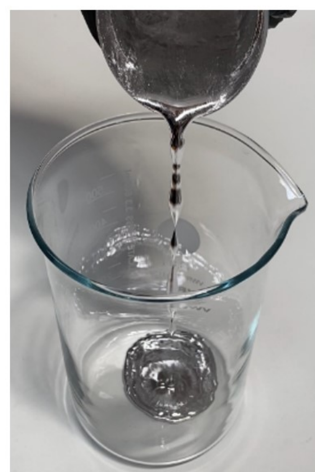
Fig. 3 - Testing the compatibility of liquid metal for magnetic heat pump. Read more at: K. Rajamani et al., ACS Omega, 49027-49036, 2023.
